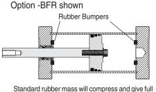
Standard rubber mass will compress and give full stoke at 60 to 80 psi. This mass can be adjusted to meet your specific pressure and/or dynamic load requirements. Temperature Range (-25° to + 220°F)
