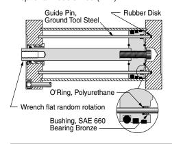
Two guide pins incorporated inside the cylinder pass through the piston head. These guide pins prevent rotation of the rod with a tolerance of  $\pm 1^{\circ}$ . The guide pins, being incorporated inside, are protected from the environment, physical damage, and are lubricated by the system lubrication, and require NO additional space, leaving the rod end area free for attachments and tooling as required by your application.
